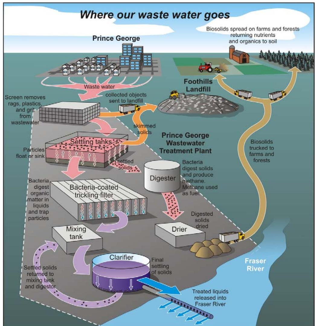
*Figure 16. A schematic drawing of a waste water treatment plant.*
